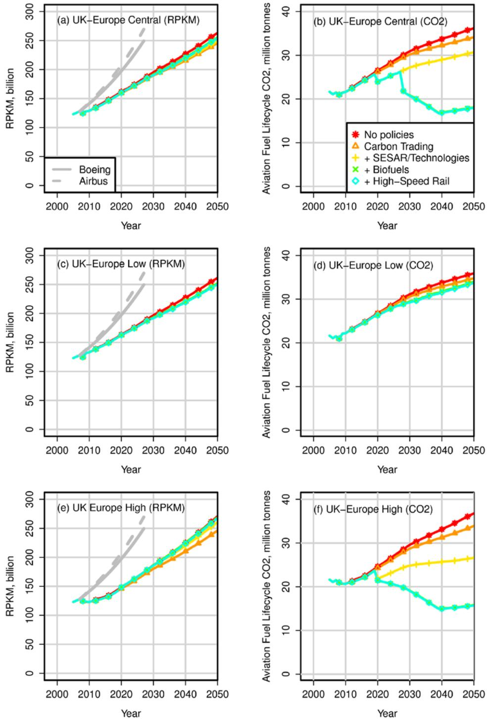
**Figure 6: RPKM and CO<sub>2</sub> emissions for international flights from the UK to the European city set modelled in this paper. For comparison, UK international CO<sub>2</sub> emissions from flights to all (global) destinations were 35.6 Mt CO<sub>2</sub> in 2006, and are projected to rise to 55.7 Mt CO<sub>2</sub> in 2050 (UK DfT central base case)<sup>46</sup>.**
