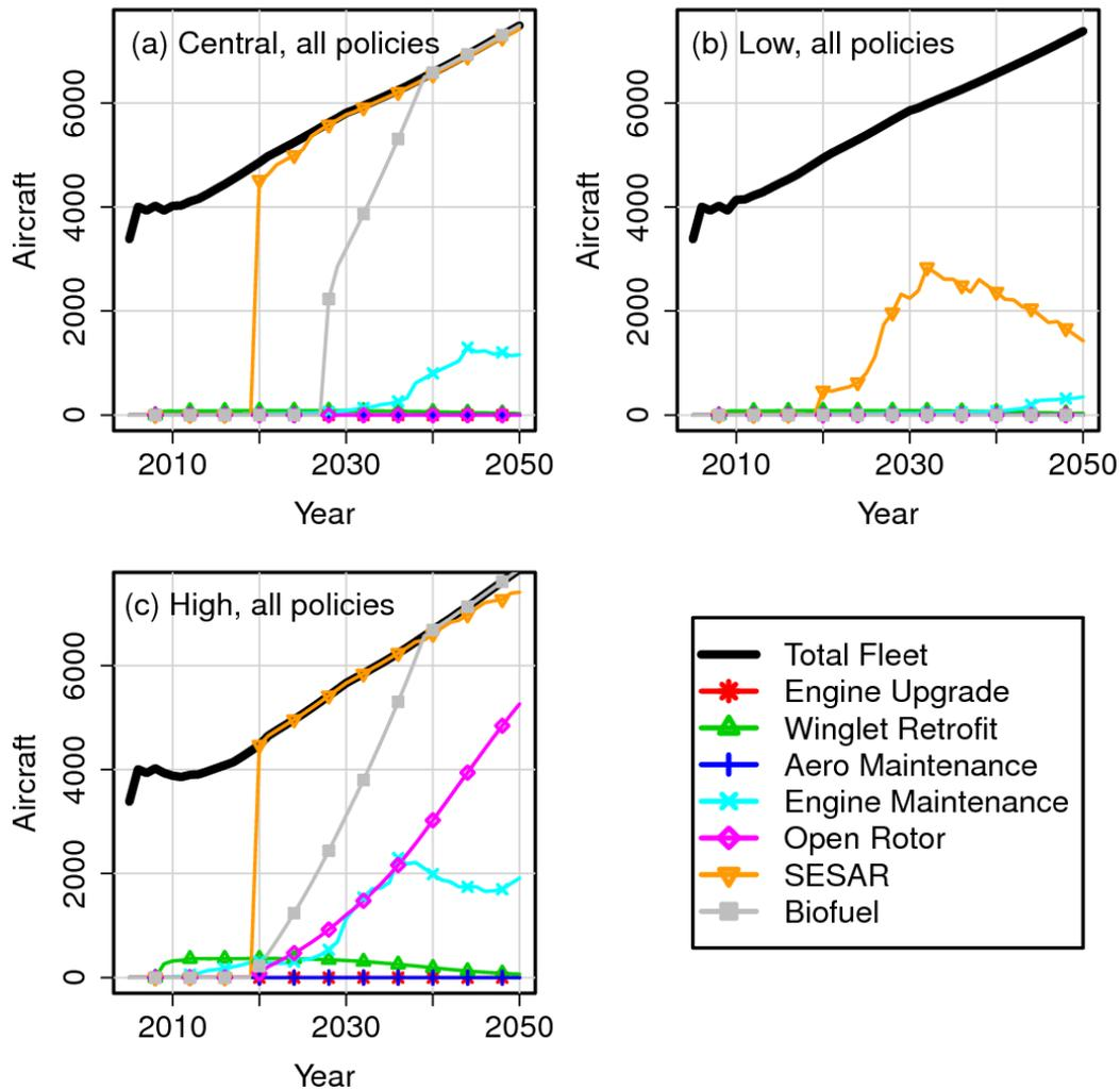
**Figure 4. Uptake of different mitigation measures by aircraft in the case that all policies are applied. Panels (a), (b) and (c) refer to the Central, Low and High background scenarios respectively.**
