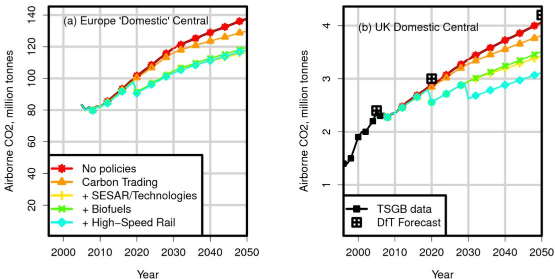
**Figure 5. Airborne CO<sub>2</sub> for the Central background scenario under different policy options. Panel (a): European domestic. Panel (b): UK domestic. Step-changes in the curves in 2020 result from SESAR, and in 2030 from the introduction of an UK high-speed rail network. The DfT forecast shown is the central base case.**
