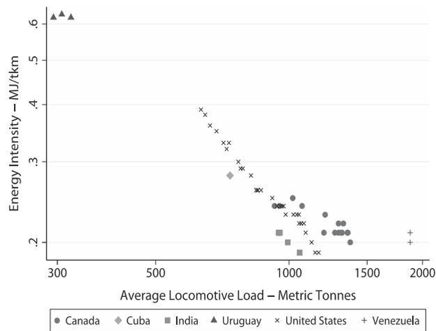
Fig. 2. Energy intensity versus average load carried per diesel locomotive for six countries.
