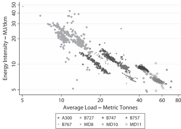
Fig. 4. Aircraft energy intensity versus average load for the aircraft types generating most tonne-kilometers operated by US carriers for 1991 to 2010. Note: Only data points with greater than 2000 departures are displayed.
