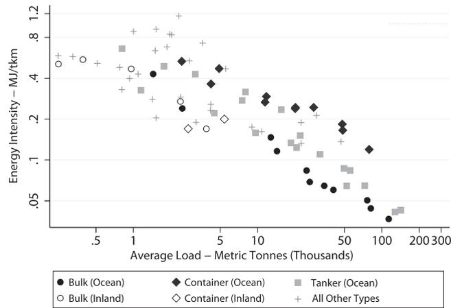
Fig. 1. Energy intensity versus average load for shipping and waterways.
