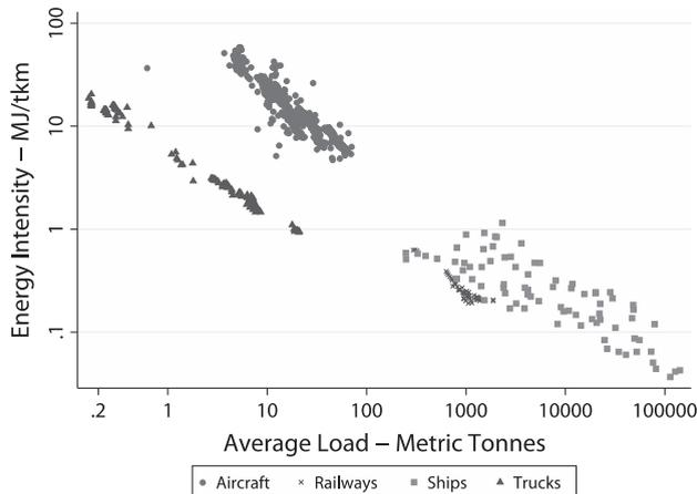
Fig. 5. Energy intensity of freight transportation modes over the average carried load per vehicle.
